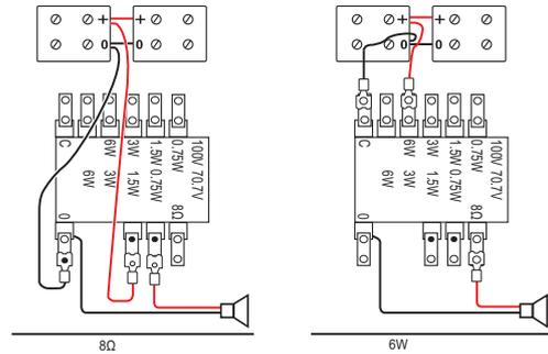
Circuit diagrams 8 Ohm and 6 W connection
