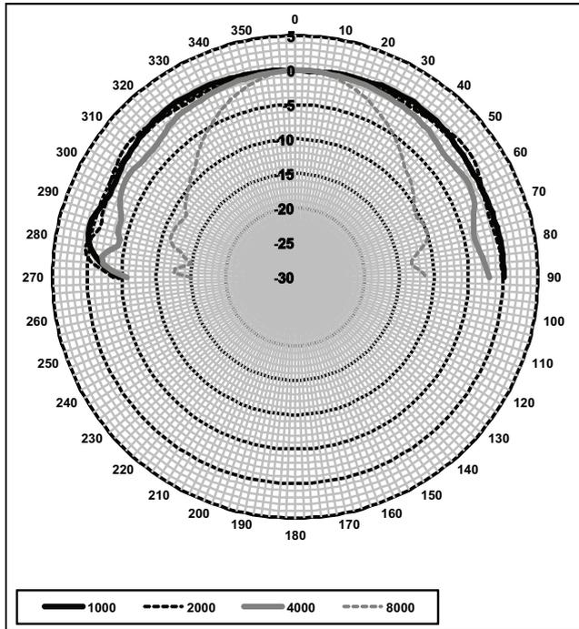
Horizontal/vertical polar diagram (high frequency).
